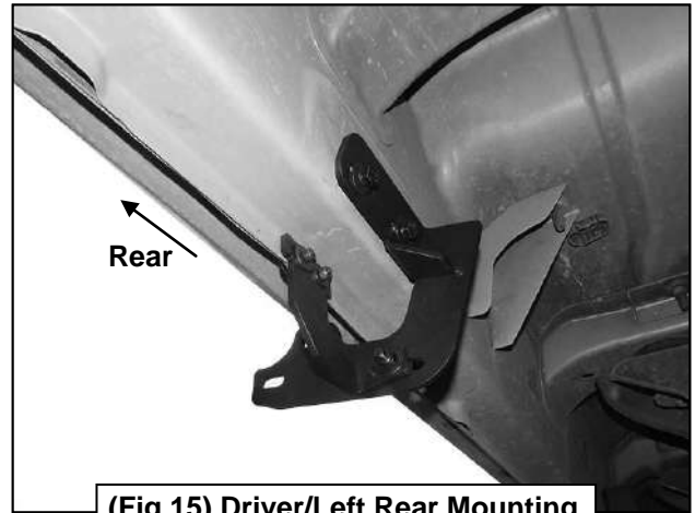
(Fig 15) Driver/Left Rear Mounting Bracket and Support Bracket attached to the rear location
