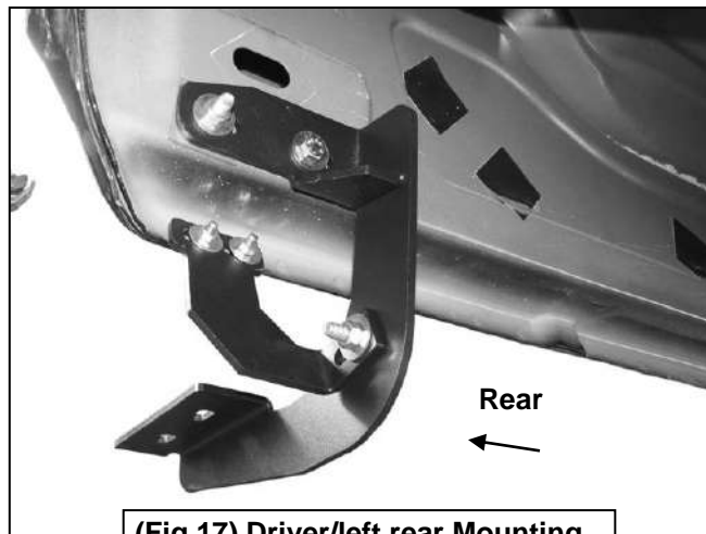
(Fig 17) Driver/left rear Mounting and Support Brackets
