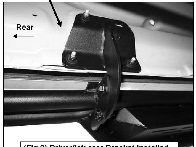
(Fig 9) Driver/left rear Bracket installed
