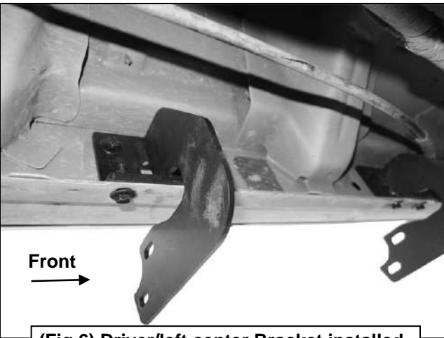
(Fig 6) Driver/left center Bracket installed
