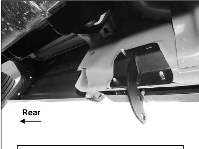
(Fig 5) Driver/Left Rear Bracket installed
