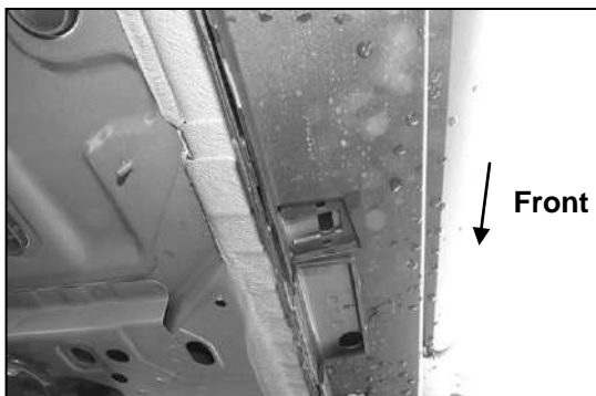
(Fig 3) Plastic clip removed from the front location trim (Passenger side shown)
