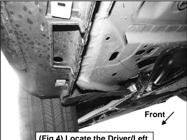
(Fig 4) Locate the Driver/Left front mounting location
