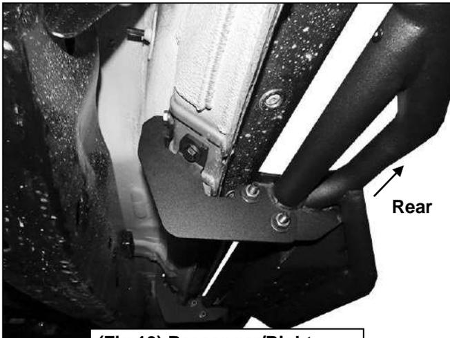
**(Fig 10) Passenger/Right Rear Running Board installed**
