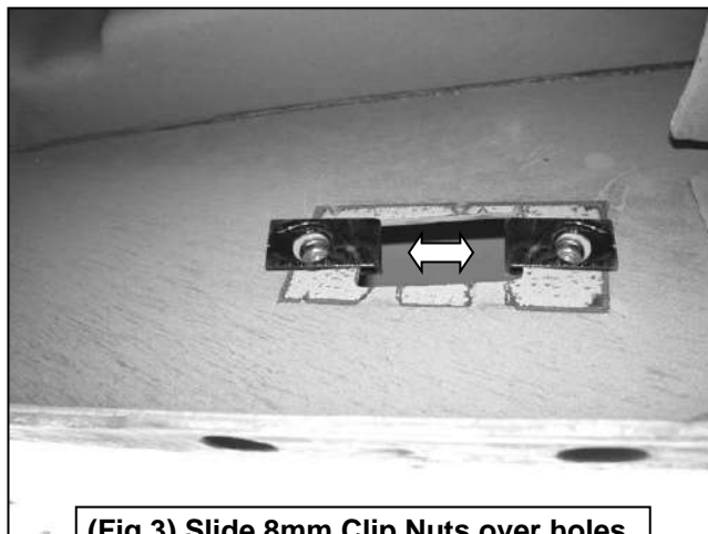
(Fig 3) Slide 8mm Clip Nuts over holes
