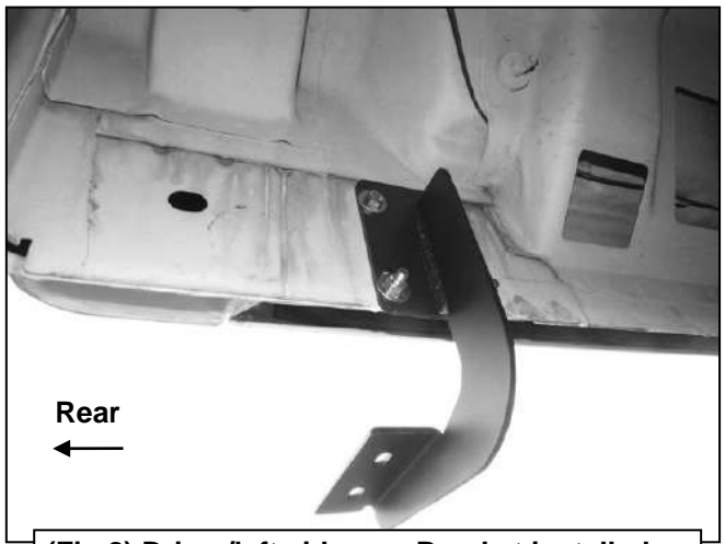
(Fig 8) Driver/left side rear Bracket installed
