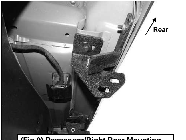
(Fig 9) Passenger/Right Rear Mounting Bracket and Rear Support Bracket attached to the rear location
