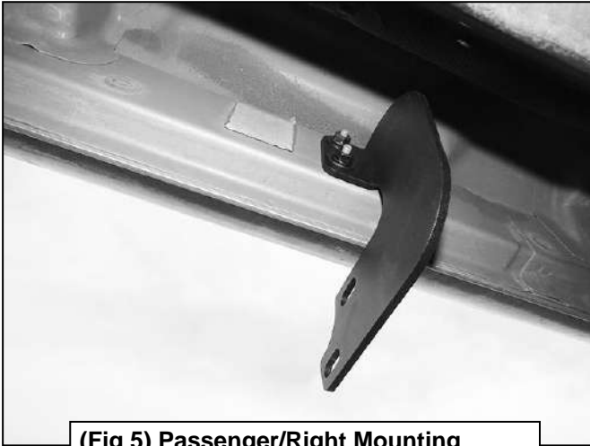
(Fig 5) Passenger/Right Mounting Bracket attached to the center location
