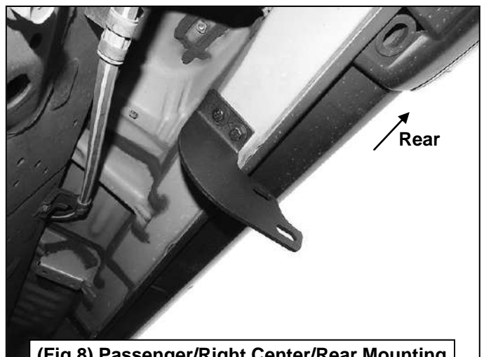
(Fig 8) Passenger/Right Center/Rear Mounting Bracket attached to the rear location
