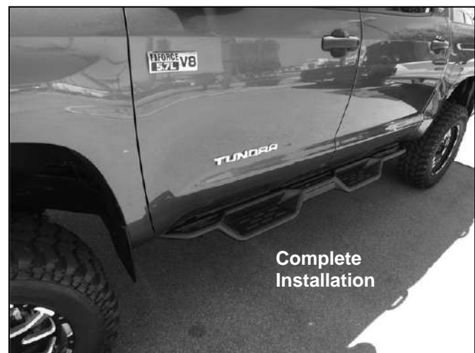
(Fig 13) Driver/left side Running Board attached to the front facing side of the front Bracket
